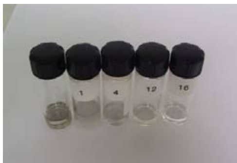
Figure 3 | The enzyme horseradish peroxidase (HRP) slowly degrades carbon nanotubes at 4 C over a 16-week period. Samples taken at weeks 1, 4, 12 and 16 become more transparent as the study progresses, which indicate the carbon nanotubes are being degraded. [Courtesy of the University of Pittsburgh]
